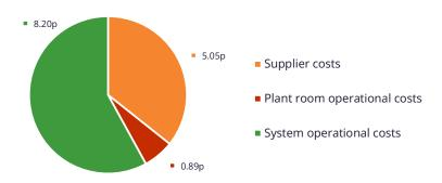
The average operational costs for a heat network equates to 56% of the unit charge breakdown.
