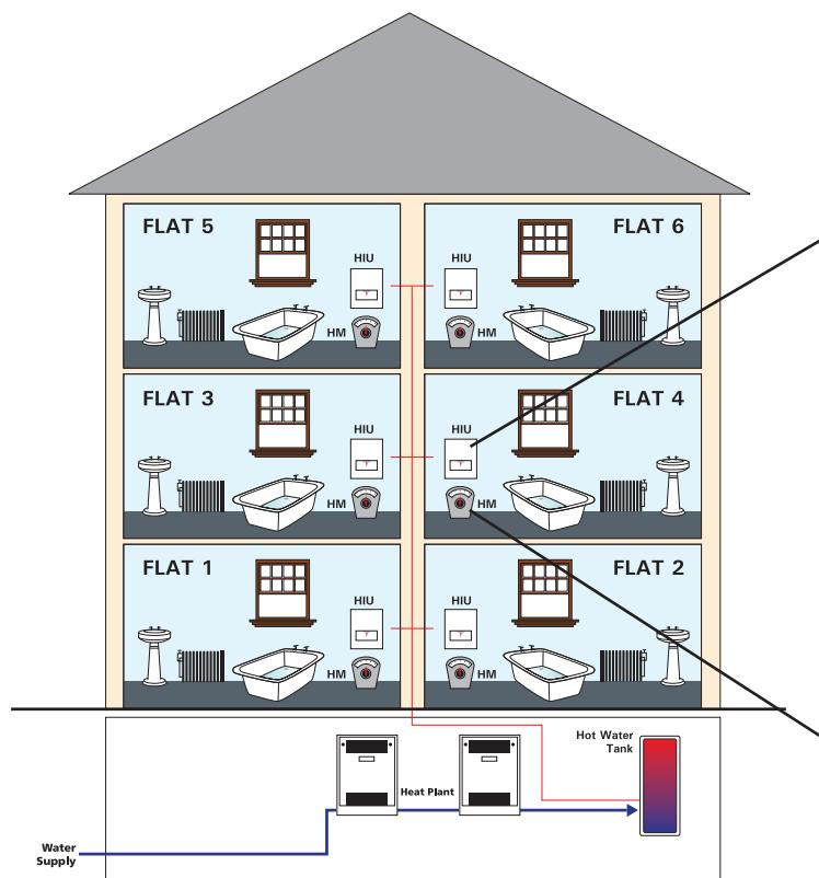
HIU = Heat Interface Unit; this unit is installed in place of a gas boiler. It takes heat from the site heat network and heats up your own heating circuit & cold water feed to give you heating & hot water on demand.
