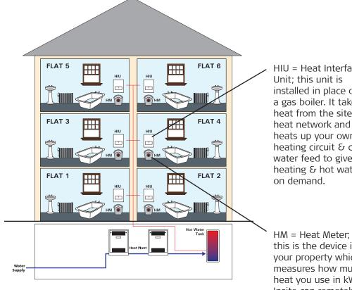
HIU = Heat Interface Unit: this unit is installed in place of a gas boiler. It takes heat from the site heat network and heats up your own heating circuit & cold water feed to give you heating & hot water
