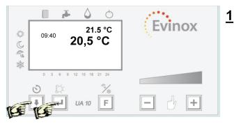
Press and hold 'ENTER' and the 'Down Arrow' button together for more than 3 sec
