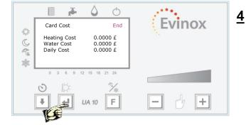
Scroll through using the 'Down arrow' until 'end' is highlighted and press 'ENTER' to exit the screen
